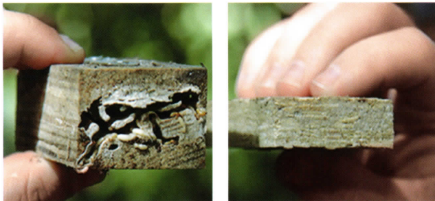
Untreated wood devastated by Formosan termites (left) and undamaged LP SmartSide product protected with the SmartGuard® process (right) during same testing period.
